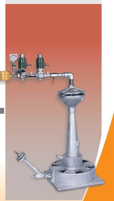
EQA 93 gas burners are used in those systems where the available pressure is 0.2 to 3 kg/cm3 and where the energy produced by the gas itself is the one necessary for its operation; that is to say, a fan or compressor are not required. When passing through the venturi, the high-pressure gas flow sucks up the necessary air for combustion, which at the same time is controlled and regulated by the primary air register.
