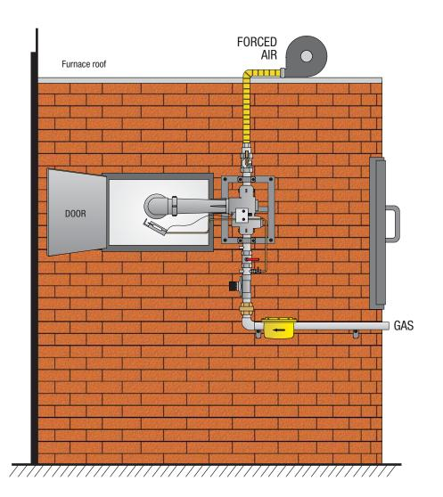
NOTE: The air and gas valves should be aligned as much as possible to allow the turn of the burner.
